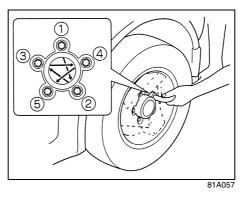
Wheel tightening torque 140 Nm (103.3 lb-ft, 14.3 kg-m)
